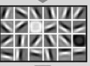
Layer 2: The computer learns to identify edges and simple shapes.
