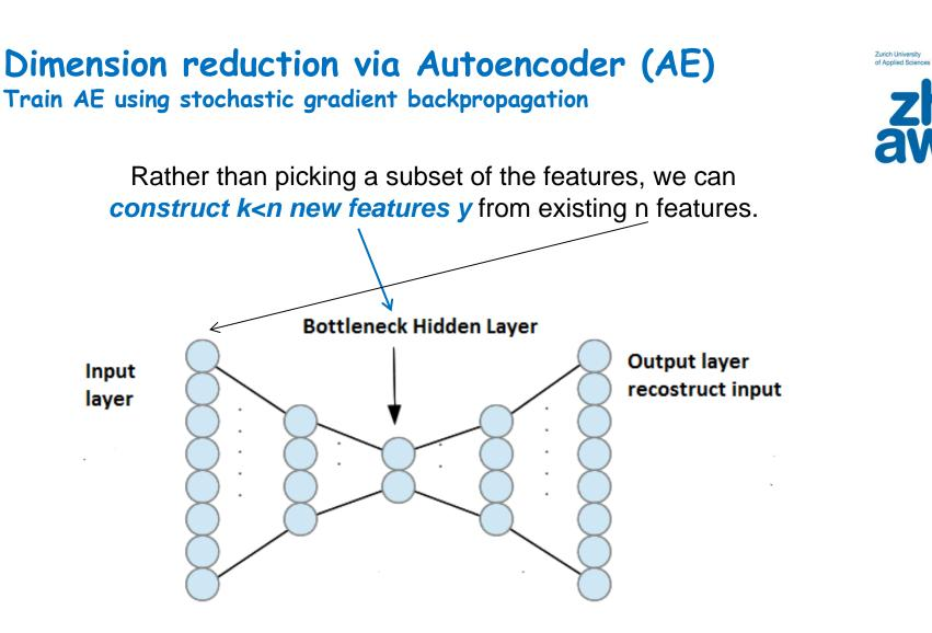
The AE network gets the optimization task to reconstruct the input which requires that essential information is represented in only few dimensions corresponding to the number neurons in the bottleneck.
